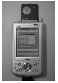
Figure 4. The CF-card RFID reader mounted on a PDA.
